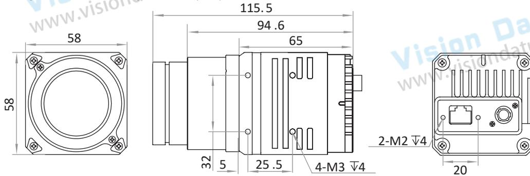
Fig. 1-1: Mechanical Dimensions (in mm) of the GigE Cameras with 6.3mm/35mm focal length lens housing (The installation uses M2 and M3 screws).
