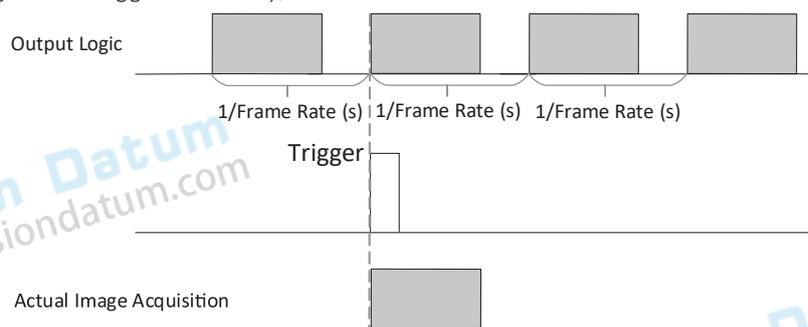
If the device receives the trigger signal during the output of each frame of image, the device will acquire images at the next frame,(uses the rising edge as the trigger activation), as shown below:
