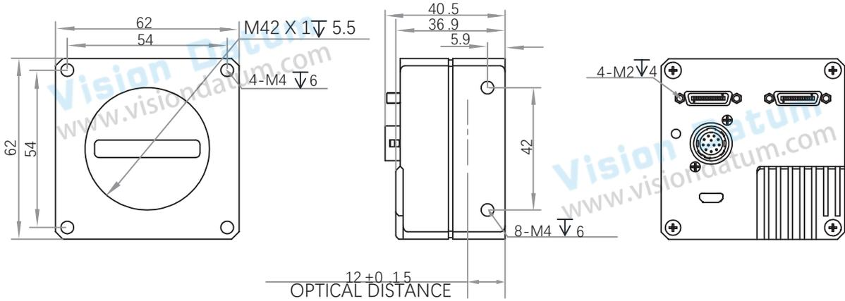
Fig. 1-1: Mechanical Dimensions (in mm) of the M42-mount 4K Cameralink Line Scan Cameras with 62 \* 62 \* 36.9 mm.
