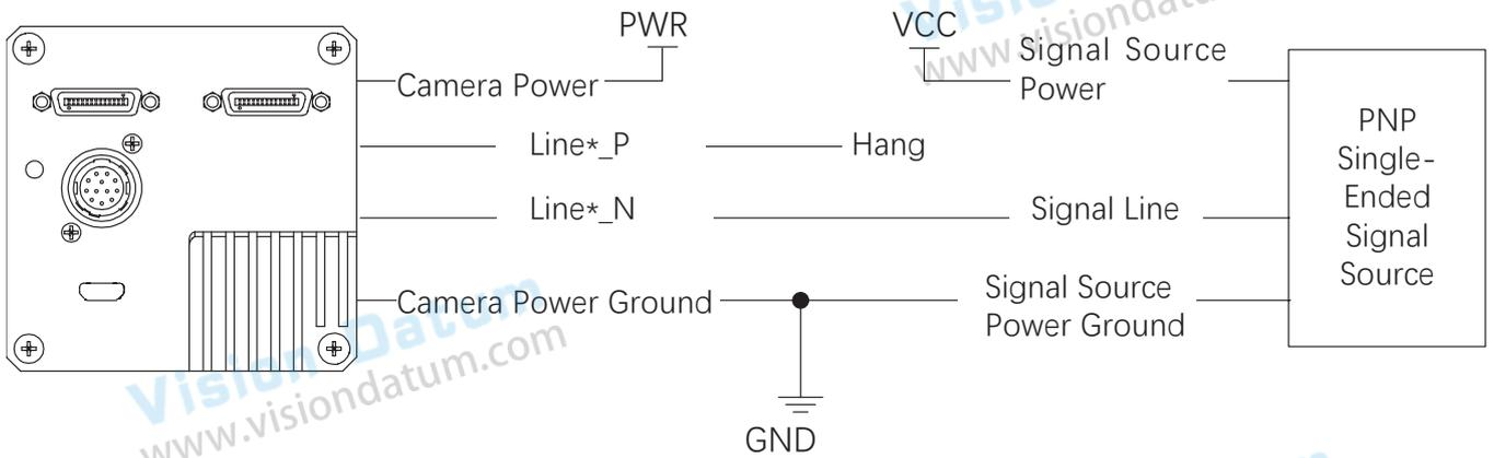
PNP Single-Ended Input Wiring with Pull-Down Resistor, the resistor range is between 1 K $\Omega$  and 4.7 K $\Omega$  :
