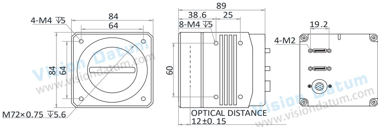
Fig. 1-4: Mechanical Dimensions (in mm) of the M72-mount 8K Cameralink Line Scan Cameras with 84 \* 84 \* 89 mm.
