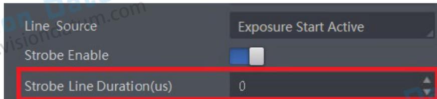
When the Strobe Line Duration value is 0, the strobe duration is equal to the exposure time.
