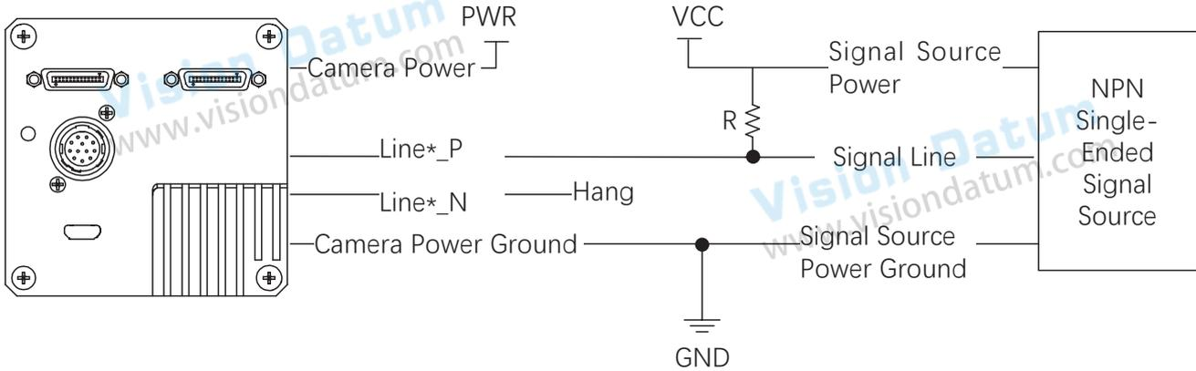
A pull-up resistor is required:
