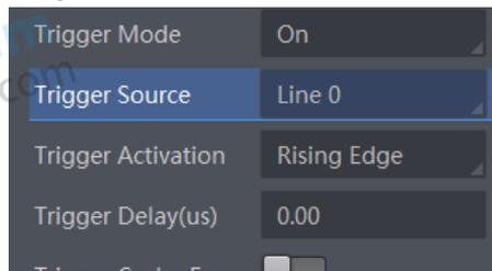
When selecting bi-directional configurable line as the hardware trigger source, you need to make sure that its line mode is input. Go to 'Digital IO Control', select specific line as 'Line Selector', and 'Input' as 'Line Mode'.
