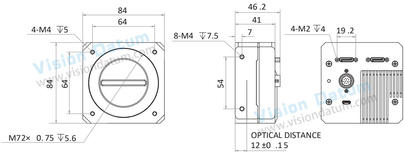
Fig. 1-3: Mechanical Dimensions (in mm) of the M72-mount 8K Cameralink Line Scan Cameras with 84 \* 84 \* 41 mm.
