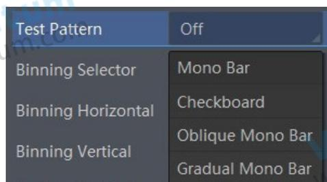
After setting the Test Pattern, the image displayed in the preview window of the frame grabber software is switched to the test image, and the specific test image is determined by the test pattern.
