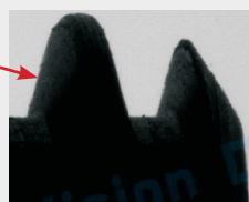
Generic Flat Lighting (BFC series) Image of screw thread and enlarged view
