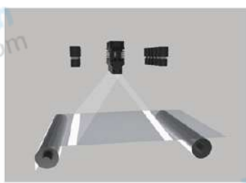
Schematic diagram of single-oblique light distribution
